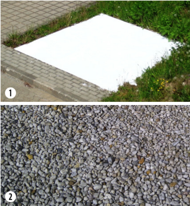
FIGURE 5: Ground surface albedo test: 1) white painted concrete 2) white gravel
