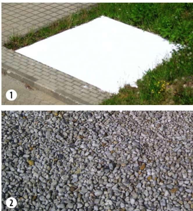
FIGURE 4: Ground surface albedo test: 1) white painted concrete 2) white gravel
